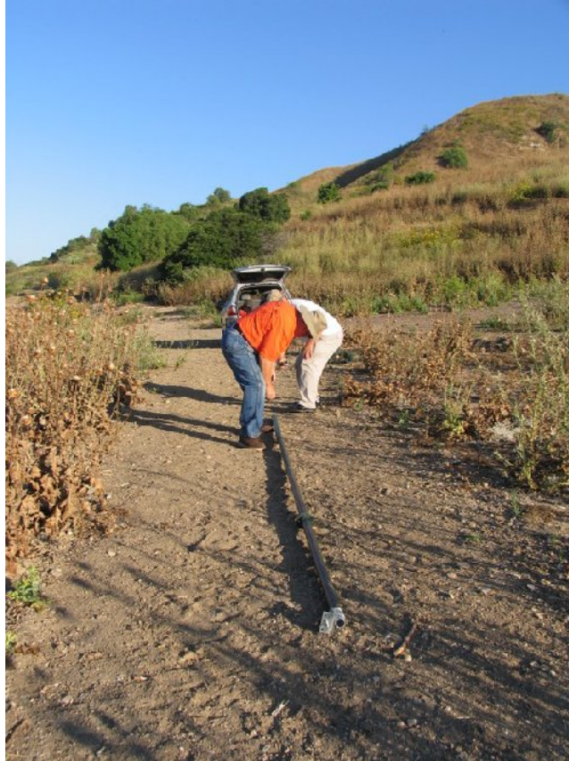
Putting the sections together. These military masts are aluminum and were originally used to hold camouflage netting.
