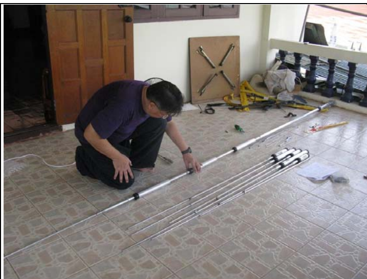
At (E20NXT) assembles the Diamond CP6A's vertical traps. He is the sponsor the Nan Repeater.
