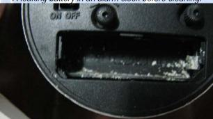
The battery compartment and terminals before cleaning
