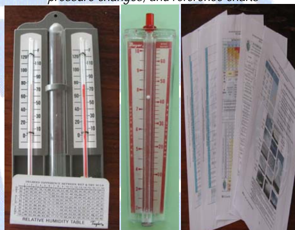
Back up: hygrometer, Dwyer wind gauge and various reference charts
