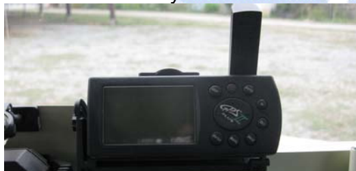
Garmin II GPS Unit Latitude, Longitude, Altitude, Date, Time, Azimuth
