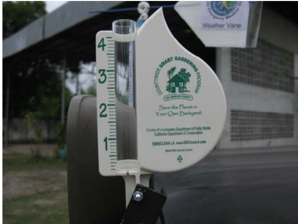
Roof mounted rain gauge
