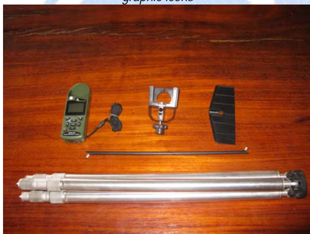
Kestrel 4500, a handheld portable fully integrated weather station
