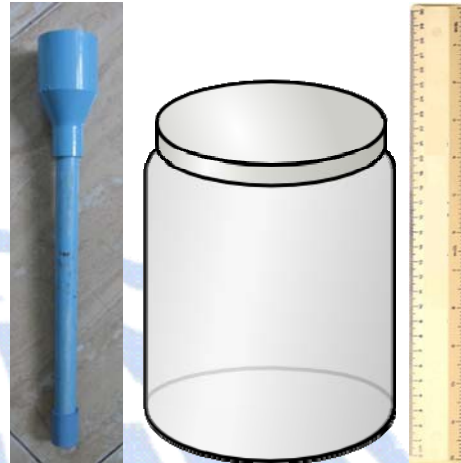
Back up: post mounted rain gauge or empty jar and ruler
