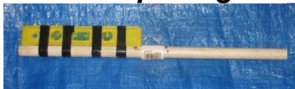
This simple spirit level on a stick with a tape measure makes slope measurements fast and easy.
