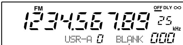
"BLANK" appears in the memory name area until [MW] is pushed for 1 sec.
