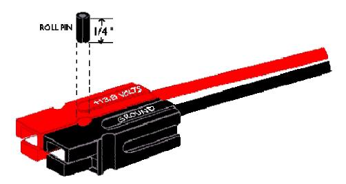
Housings should be mated according to the diagram above, viewing from the contact side (opposite the wire side), tongue down, hood up, RED on the LEFT, BLACK on the RIGHT. Use a 3/32-inch-diameter roll pin, 1/4 inch long, to keep the housings from sliding apart.
