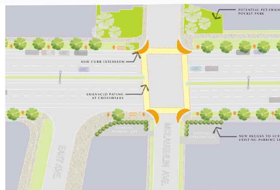
PROPOSED CORNER CURB EXTENSIONS along Venice Boulevard create a safer crossing for pedestrians by reducing the length of the crosswalk. Enhanced crosswalk paving at these intersections clearly mark the major pedestrian circulation paths.
