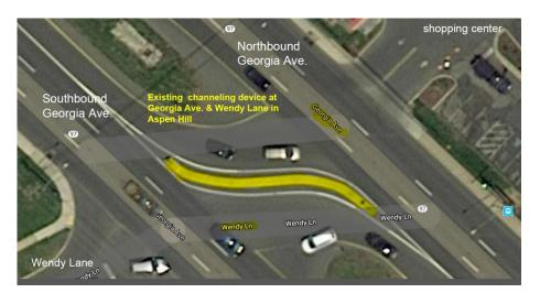
An existing example of such an intersection is Georgia Avenue and Wendy Lane in Aspen Hill. The device prevents going straight through the intersection or turning left from the secondary road/shopping center onto the main road. Traffic on Georgia is able to U turn or turn into secondary roads.
