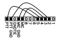
Radio Shack® RJ45 (8 wire) Modular mic. connector radios HTX242 etc., FM radios
