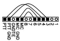
Typical Yaesu® RJ45 (8 wire) Modular mic. connector radios Most but not all FM rigs. including FT817,FT897,FT857
