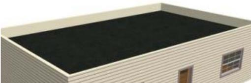
A flat roof showing the extension of a parapet
