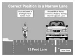
into the right-hand vehicle track should cause motorists to move into the adjacent lane to maintain the required separation.
