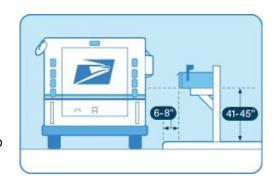
Post mounted mailboxes— the support should be secure and safe. The best supports are designed to bend or fall away if a car hits them.
