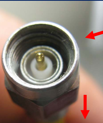
SMA Male to fit SMA Female on Radio
