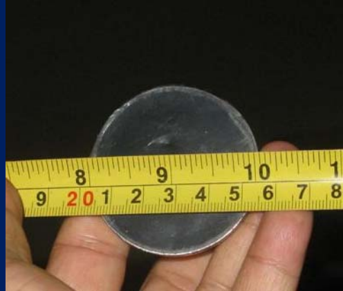
The Button magnet total surface area: 19.63 sq cm / 3.14 sq in.
