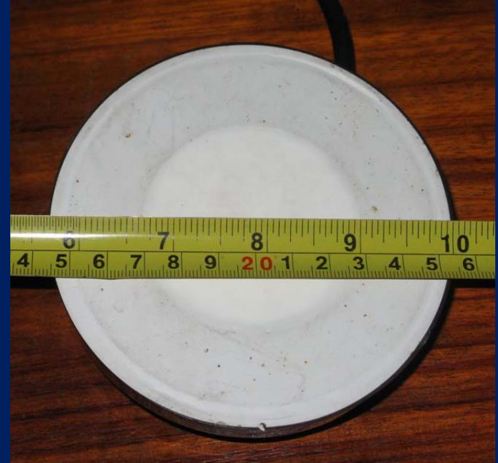
The NMO magnet total surface area: 86.59 sq cm / 15.9 sq in.
