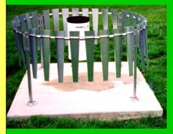
If put on the ground, the top of the rain gauge should be 50 cm above the ground.
