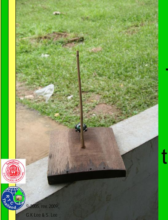
Step 1. Put the Wind Tell "Tail" in an open area where the wind can blow on it.
