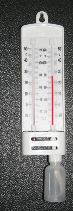
The thermometer must be in the shade. It should be 1.5 m above the ground.
