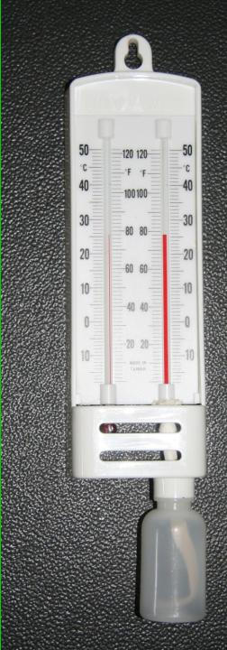
You can use the dry bulb thermometer on the hygrometer.
