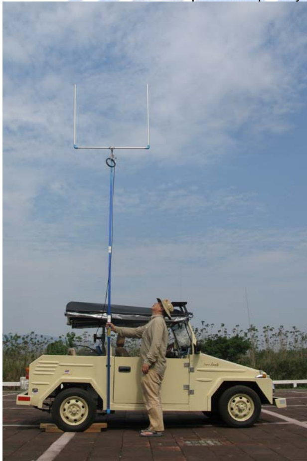
The Slingshot beam at max mast height: tip of elements is 5.16 m AGL; feed point at 3.86m AGL.
