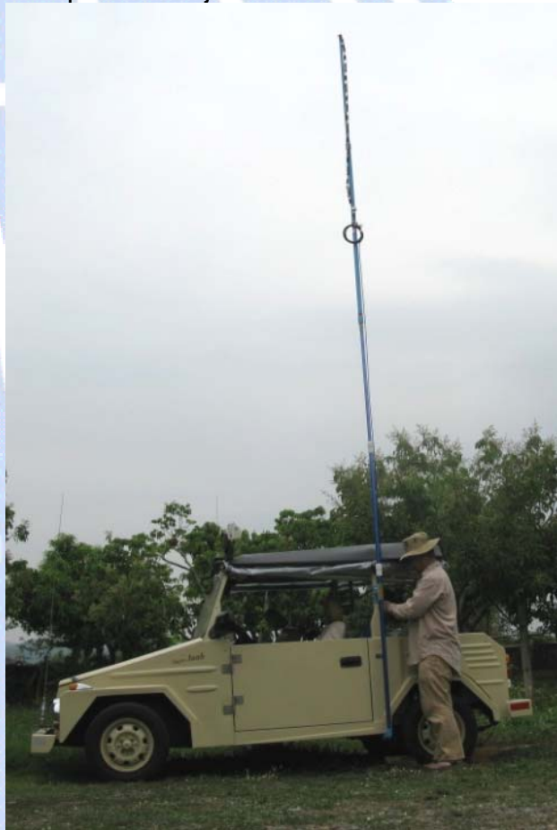
The 450 Window Line Slim Jim at max mast height: tip of antenna at 5.85m AGL; feed point at 4.35m AGL.
