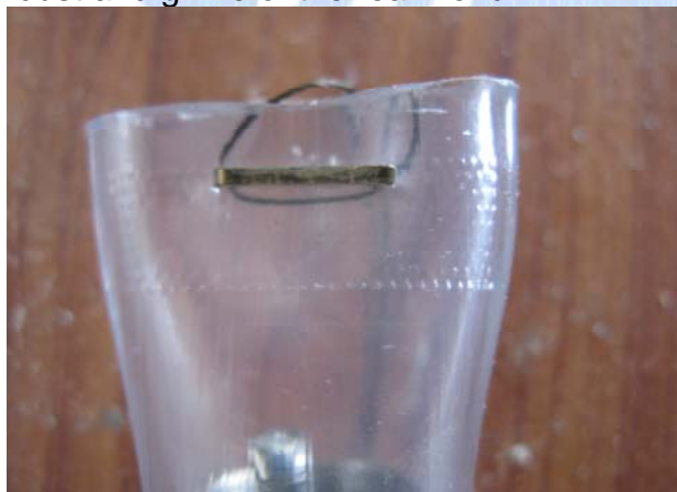
The tether is looped around the staple..
