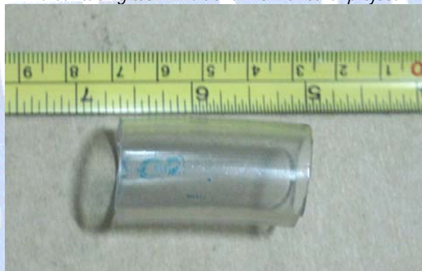
Cut the tubing to 1 1/2" lengths and ready for stapling.
