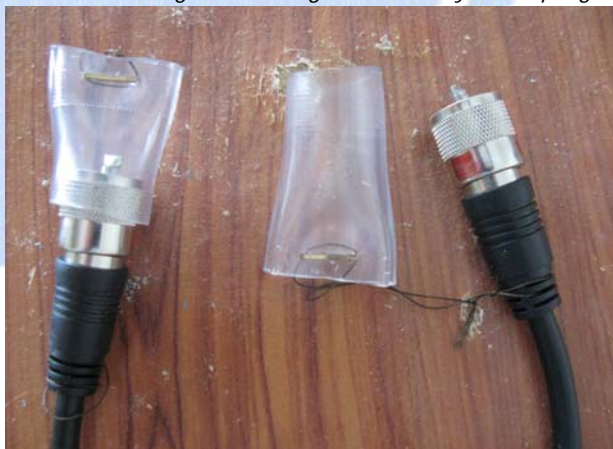
Dust cap on (left) and off (but tethered) on the PL-259..
