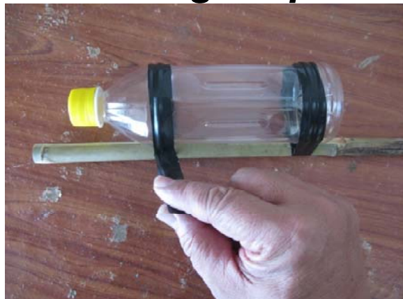
A leveling stick is easy to make: a straight bamboo stick, and empty water bottle, and some tape.
