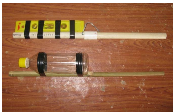
Two leveling sticks: spirit level and water bottle versions. A stick length of 0.5m makes them more portable (if 1m long = no calculation need).
