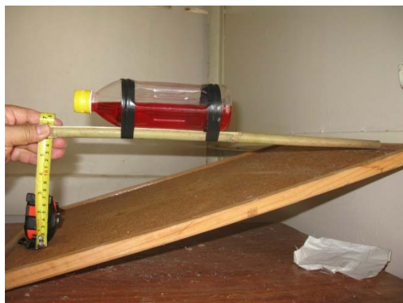
It's also easy to use. Plain end of stick uphill; bottle end downhill. Raise bottle end until water is level. Measure from bottom edge of stick to ground in cm. Multiply the distance by 2 = % slope. In the photo, 15cm = 30% slope for the demonstration.
