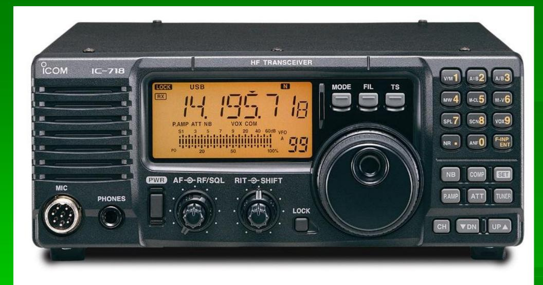
Can you find the "up" and "down" controls, the Squelch control, the Shift control, and the RIT control on this transceiver? The tuning Step control?
