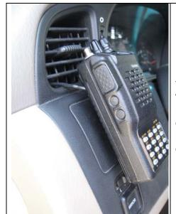
The end result is a very neat radio mount with no loose wires an no obstruction of the dashboard controls, instruments or displays.
