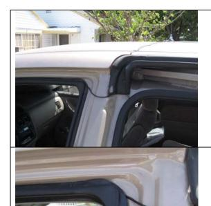
The "kiss" magnetic mounted antenna for the VX-150 was placed about the center of the roof of the Honda Odyssey mini-van.
