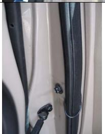
I hid the coax behind the door gasket all the way to the front edge of the door window, and half way down the front edge of the door. Excess coax was looped back up the front edge of the door on the inside door gasket.
