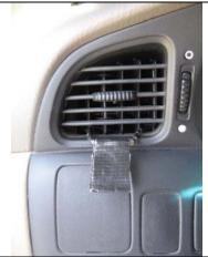
A wire hook / loop was made to secure the VX 150 to the ventilation grid, yet not interfere with the dashboard controls or instrument cluster.
