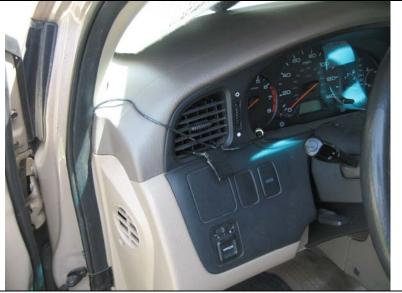
The coax emerges from behind the interior front door gasket at the top of the dashboard. There is sufficient coax remaining to allow for connecting / disconnecting the VX 150.
