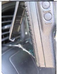
The VX 150 belt clip captures the hook / loop on the ventilation grid to secure the radio to the dash.
