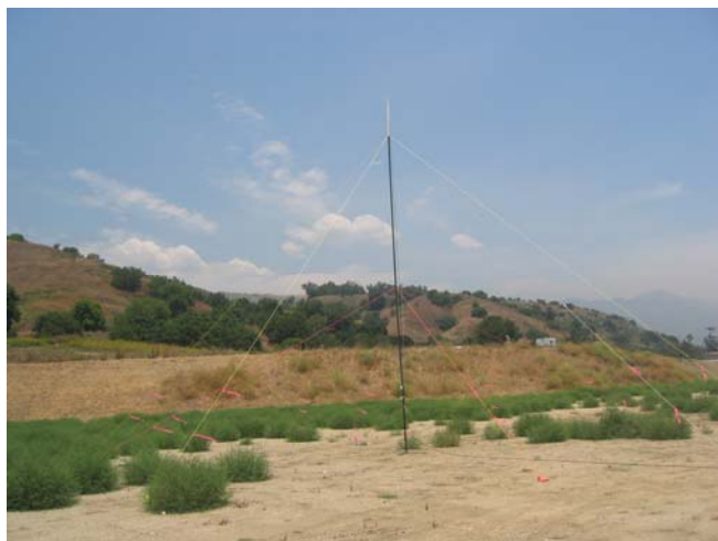
40 Meter Inverted V Dipole built by Mark KF6DSA
