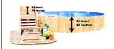
3/ PERIMETER BARRIER AND GATE. All swimming pools must have a barrier around the perimeter of the pool that prevents access. The barrier must completely surround the pool and the top must be at least 48 inches above grade at all points. This requirement also applies to the gate that limits access to the ladder or steps
