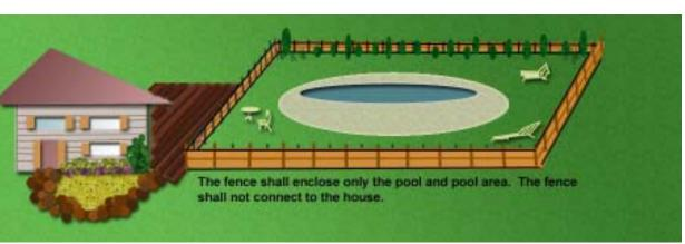
unit. The house <u>shall not</u> be used as a barrier for any portion of the area surrounding the pool.
