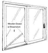
installed in the upper track will prevent windows from being lifted up and out or their tracks.
